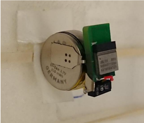
Figure 37: A tiny ANNA-B1 application including coin cell battery with the range of about 100 m, size 7.5 x 12 mm
