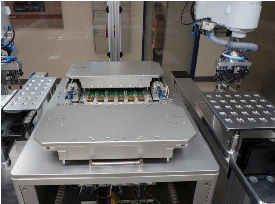
Figure 26: Automatic test equipment for module test
