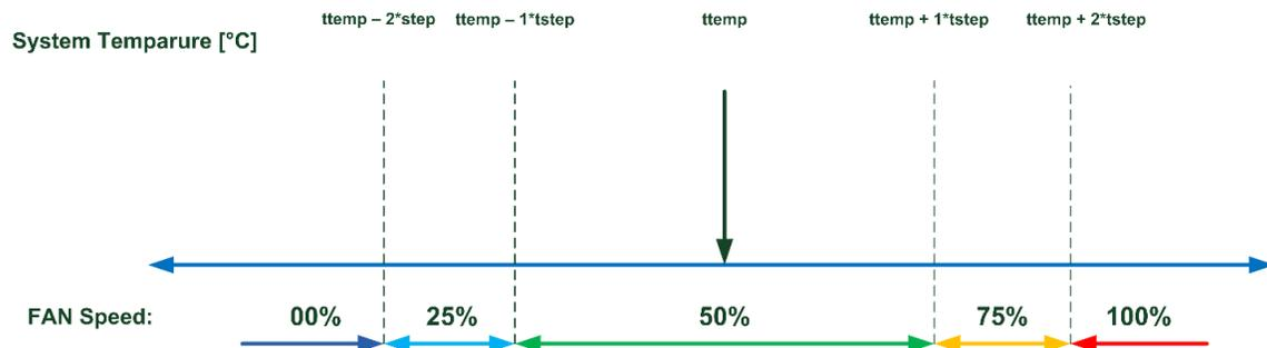
The user can change the ttemp to any value, effectively moving the window up or down in the temperature scale.
